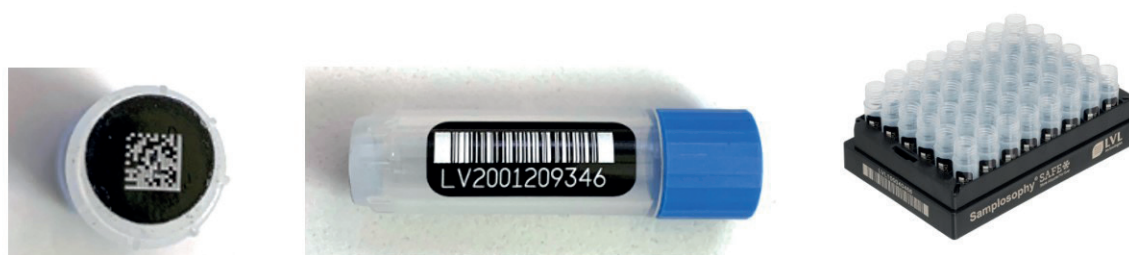
Figure 4 Cryotubes with a unique 2D barcode for long-term storage of serum and plasma samples.
